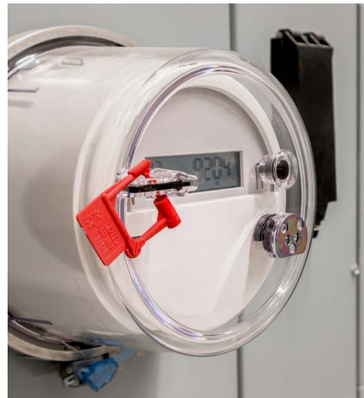
Smart Utility Meter
