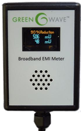
Many people want to know how effective Greenwave-SOLS filters are at reducing the dirty electricity flowing along electrical wiring in their homes and other places. This is easy to measure with a plug-in dirty electricity meter, such as the *Greenwave Broadband EMI Meter* shown here.
