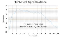
Frequency Response:  $650MHz - 10GHz(\pm 6dB)$ Full Frequency Response: 200MHz - 12GHz Response Time:  $< 5\mu s$
