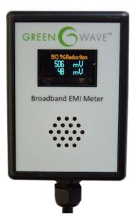
Greenwave's meter is easy to use. Simply plug it into electrical outlets to find out how much dirty electricity is present on nearby wiring. The meter can show "BEFORE filter" and "AFTER filter" measurements on the same screen simultaneously, making comparisons easy.
